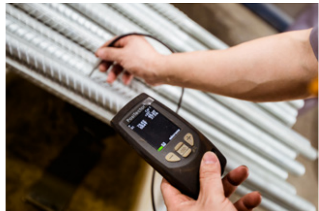
Control of coating thickness
