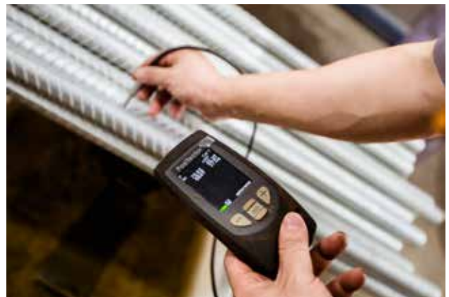
Control of coating thickness
