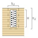
ALUMINI with SBD self-drilling dowels
