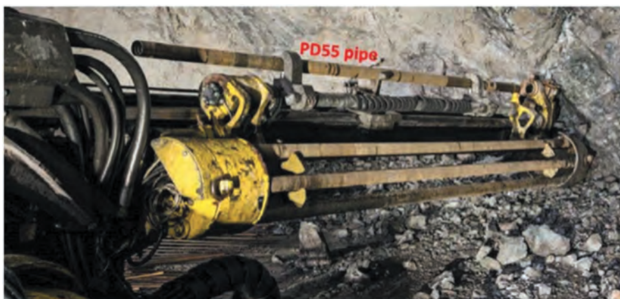
Figure 2. Rod magazine Atlas Copco Sandvik with PD55 drill pipes loaded.
